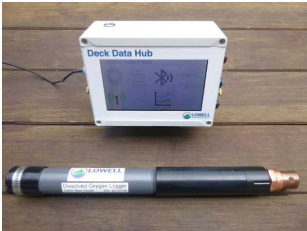
Figure 1. Data deck hub box and a dissolved oxygen / temperature logger (image courtesy of Lowell Instruments).
