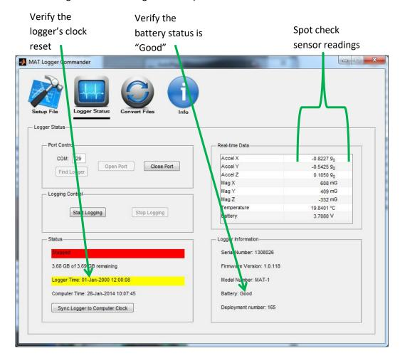
IMPORTANT: You are not done yet. Perform a battery test run to test for, and to remove, passivation of the lithium metal battery before starting a field deployment (see below).
