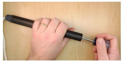
3. Gently pull the end cap up and out of the top of the carbon fiber housing.
