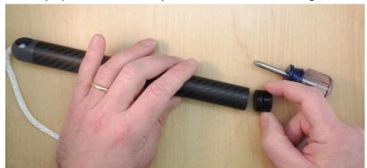
4. Remove the "X" spacer from the housing.
