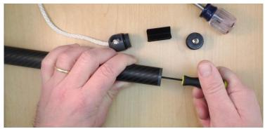
7. The board should now be loose within the housing. Use the 3/4" dowel to gently push the circuit board and logger assembly out of the housing.
